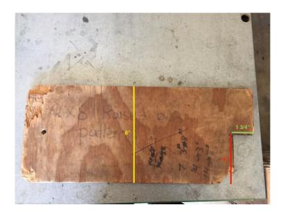
And here is a design of the Lumber with the position of the notches to give you a better idea of where the 4" and the 1 and 3/4" cuts would go on the lumber.
